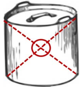
Measure at the geometric center of cooking vessel
